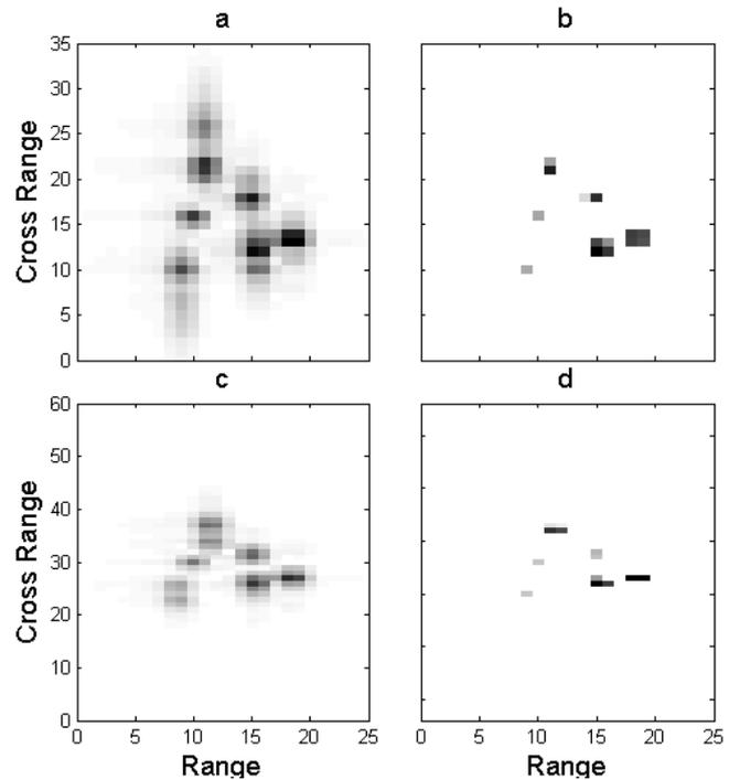
Figure 2. ISAR images from experimental delta-wing data. First column contains Fourier transform-based images and second column contains S-method-based ISAR images. Each image is zoomed in on the target for clear presentation.
