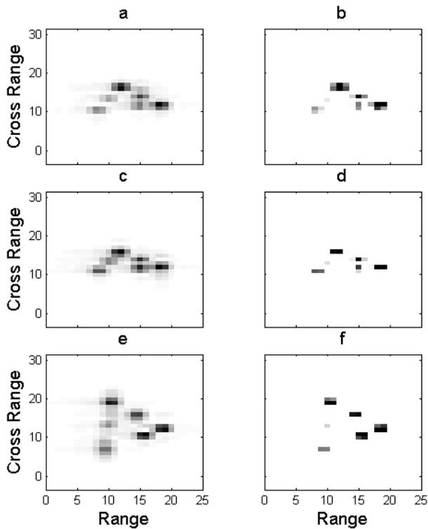
Figure 3. ISAR images from experimental delta-wing data. First column contains Fourier transform-based images and second column contains S-method-based ISAR images. Each image is zoomed in on the target for clear presentation.
