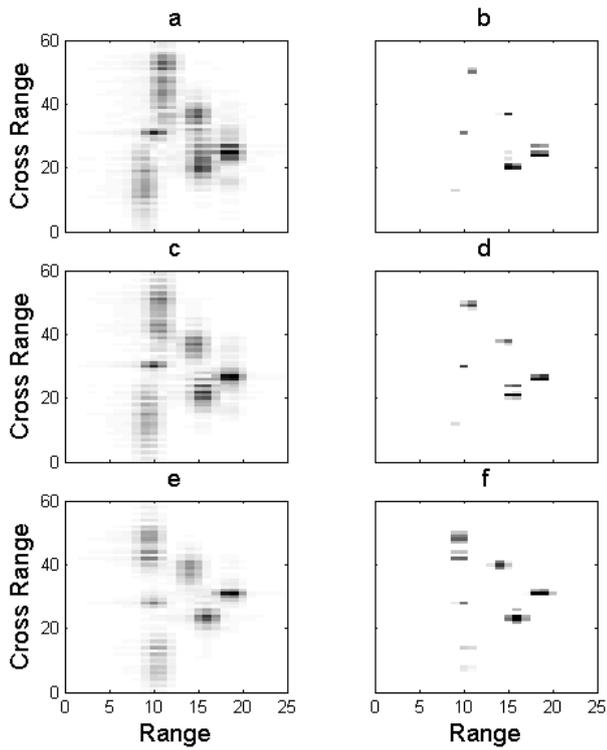
Figure 1. ISAR images from experimental delta-wing data. First column contains Fourier transform-based images and second column contains S-method-based ISAR images. Each image is zoomed in on the target for clear presentation.
