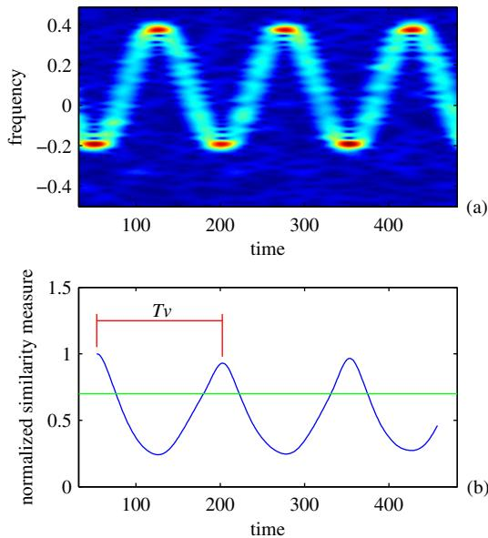
Fig. 1. Micro-Doppler period estimation in white noise environment: a)  $|STFT(n, k)|$  of the signal from the Example 1; b) Obtained normalized similarity measure
