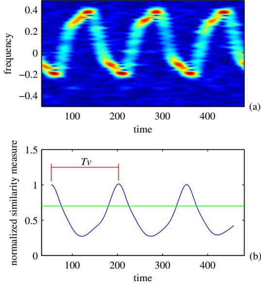
Fig. 2. Micro-Doppler period estimation in white noise environment: a)  $|STFT(n, k)|$  of the signal from the Example 2. b) Obtained normalized similarity measure
