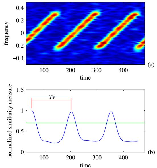
Fig 5. Micro-Doppler period estimation in white noise environment: a)  $|STFT(n, k)|$  of signal described in Example 5; b) Normalized similarity measure
