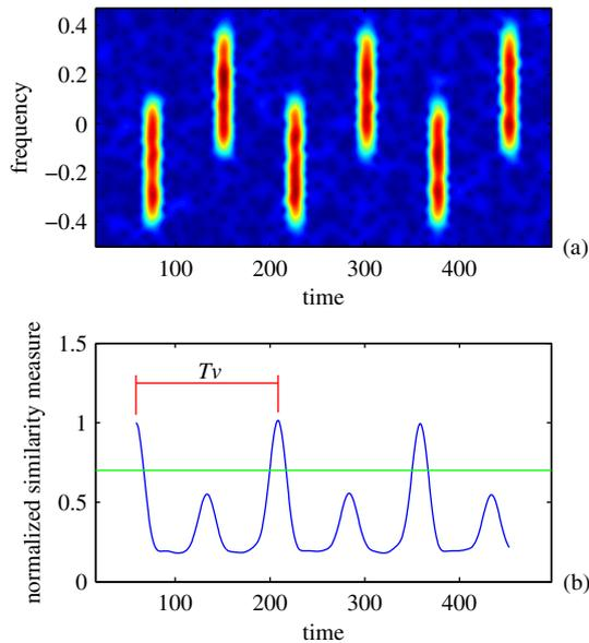
Fig 3. Micro-Doppler period estimation in white noise environment: a)  $|STFT(n, k)|$  of signal from the Example 3; b) Obtained normalized similarity measure
