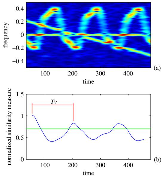
Fig 4. Micro-Doppler period estimation in white noise environment: a)  $|STFT(n, k)|$  of signal described in Example 4; b) Normalized similarity measure
