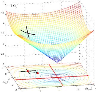
Fig. 1. Illustration of the  $L_1$ -norm and its gradient with two missing samples
